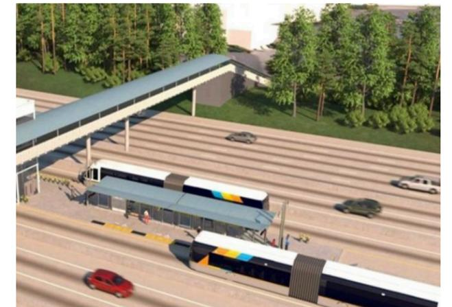
BRT in-line station concept with access from the center of GA 400.
