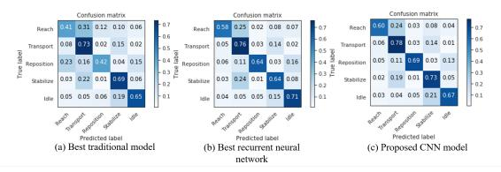
Figure 3: Confusion matrices for (a) best traditional model, (b) best recurrent neural network, (c) proposed convolutional model. From the confusion matrices, it could be seen that *idle* is confused with *stabilize* and *reach* is confused with *transport*.
