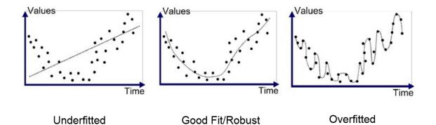
Figure 2: Left plot shows a rigid function (model) which tend to be simple like a linear function that underfits the training data. Right plot shows a flexible function (model) which tends to be more complex like a higher order polynomial that overfits the training data. In both the cases, it is easy to see that both the functions (models) won't perform well on the unseen data. Instead, a balance should be maintained between the two extremes as shown in the center plot.
