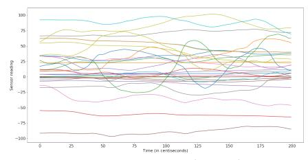
Figure 1: A sample IMU data, which is 200 time-step long (2 secs long). The plot shows several lines where each line represents how the reading of a single sensor changes over time. Such a sample IMU data which is in  $\mathbb{R}^{76\times 200}$  acts as an input to a machine learning model that identifies the primitive taking place in it.
