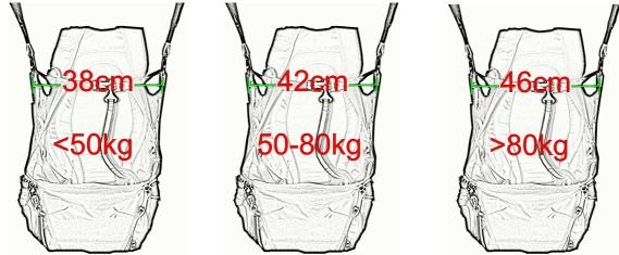
When testing in two-seater configuration the horizontal dimension of the passenger's harness is set to the same width as the pilot's harness. The pilot's weight is defined at pilot's bodyweight plus any ballast carried.
