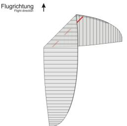
side as fast as possible to collapse the canopy asymmetrically at 50 % of the span at an angle of approximately 45° relative to the longitudinal axis. As soon as the collapse is achieved, release the lines guickly.
