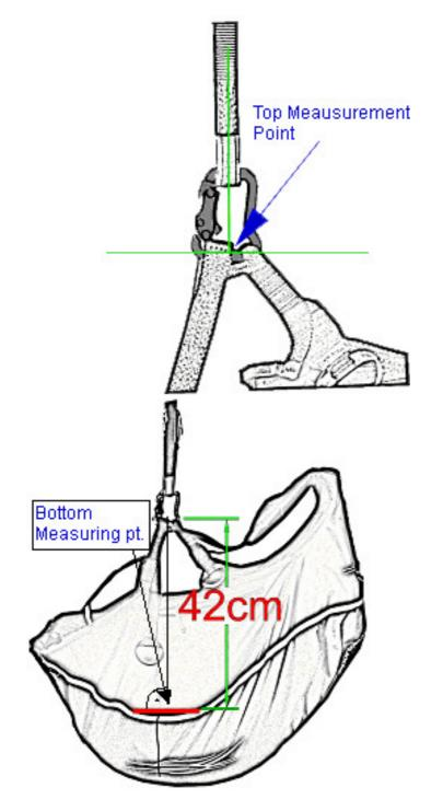
The horizontal distance of the paraglider riser attachment points (measured from connector centrelines) shall be set to 42 cm.
