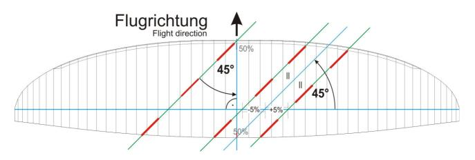
Note: all measurements are given as percentages of the flat span of the paraglider.
