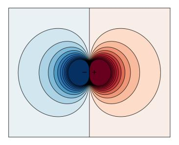
So... if you design a dipole using a coaxial woofer where the tweeter is a Constant Directivity horn – and if you add a CD horn tweeter on the back to make back and front symmetrical – you get a true Constant Directivity response both front and back. The dipole configuration automatically makes the woofer into a Constant Directivity source.
