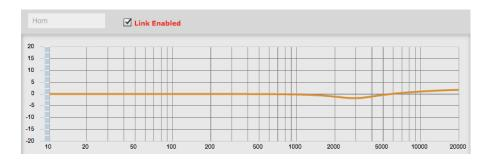
On the back is a PRV WG175PH horn tweeter. Its response is similar enough to the Radian Coaxial for my purposes. An L-Pad lets me turn it up louder, or turn it completely down. This curve is when set at 3 o'clock.
