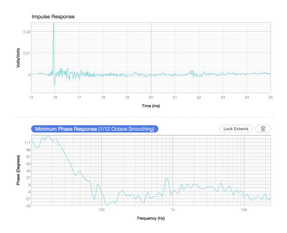
Impulse response should look like an upside-down T, and it does, with only a touch of overhang. And as you can see, the phase response is +/- 45 degrees from 40 Hz to 25 KHz with no polarity reversals or phase rotations. 99.5% of speakers would butcher the impulse. 99.5% of speaker designers ignore phase response and only give a shrug to impulse response.
