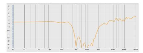
Which is combined with an 18dB/octave IIR filter to finish what the FIR filter couldn't...
