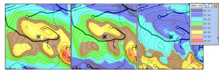
Figures above show calculated wind resource maps. To the left WASP, in the middle CFD, and to the right the compare layer (WASP minus CFD). As shown, up to a 0.7 m/s higher calculation value by WASP than by CFD. Without the compare layer it would be hard to evaluate the more precise differences between the two models. See also graph at the end of next page.
