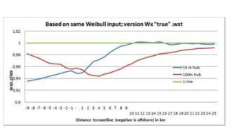
Calculated Energy output with WASP 10.2 (same as WASP 11) relative to WASP 9. Up to round 6% less can be seen in this specific example. And it shall be noted that there is a large hub height dependency.
