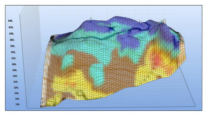
The last presentation shows the WAsP minus CFD result compare layer draped on elevation data. Here it is easy to see that it is in the valleys (areas behind hills), where the wind speeds are estimated a bit higher with the WAsP model compared to the CFD model.
